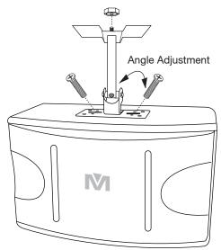
NOTE The structure of the ceiling must be strong enough to hold at least 50 pounds. The ceiling mount bracket in the diagram is Model: SPS-706 and it is optional.
