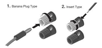
Before connecting the speaker to connection, you must make sure that the master volume and the AC power are off. Otherwise, it may burn your speaker. Then, double check the connection to match the "+" and "-" correctly.
