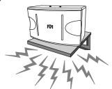
NOTE Always be sure that the surface chosen for mounting is structurally capable of supporting the weight of the speaker. Do not mount more than one speaker into one Ceiling Mounting Bracket (optional). Also, avoid having sound absorbing material such as curtains, etc. on the wall or placing the speakers too close to the window.
