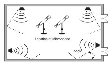
When using several speakers at the same time, special care must be taken to ensure that the output level of the speakers would match each other in order to avoid feedback which may burn the tweeter with high frequency.
