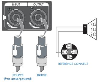
Source (INPUT) comes from the output source of the active/powered speaker while the bridge (OUTPUT) connects to the passive/non-powered speaker.
